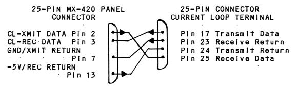
The cable should have the following internal connections:
