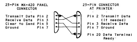
The cable should have the following internal connections:
