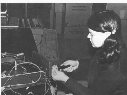
CRT displays units are in the chassis prep stage with Alsena Smith performing the operations.
