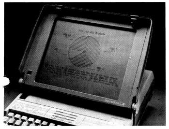
The new liquid crystal display screen (LCD) available as an upgrade for current DATA GENERAL/One models, optimizes screen polarization which substantially improves character-to-screen contrast quality.
