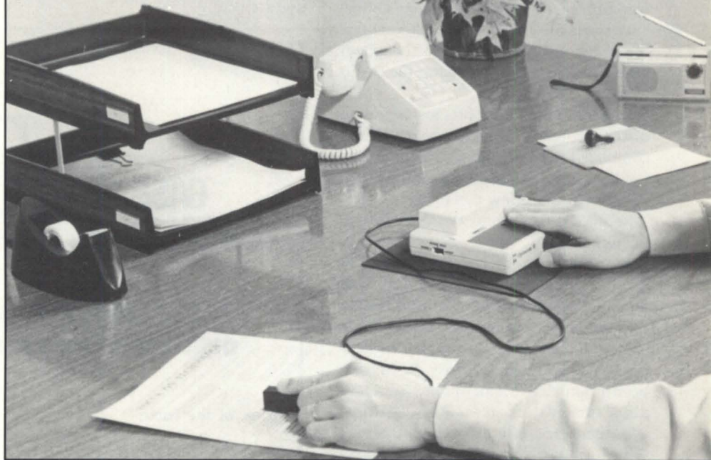
The Optacon print-reading aid from Telesensory Systems, Inc. makes printed material accessible to blind people. A small hand-held camera in one hand scans text and converts it to shapes of characters recognizable by a finger on the other hand.
