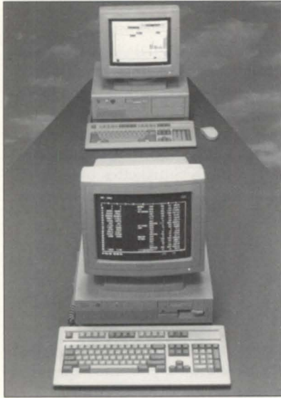
The new Dasher/386-25k (rear) supports both MS-DOS and Unix operating systems for a base price of $4,995, including 4 MB of memory and a 100-MB hard disk. The Dasher/286-12j (front), a compact, IBM-compatible system that runs MS-DOS, includes 1 MB of memory, two diskette drives, and a 40-MB hard disk, for a price of $2,375.
