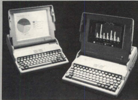
The DG/One Model 2T is available with a backlit, blue LCD screen (left), or a light-emitting electroluminescent (EL) screen with CRT-quality resolution (right).
