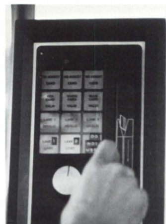
A magnetic card reader allows the transport operator to identify himself to the computer.
