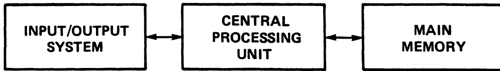
Figure 2.10 The Three Sections of a Computer System
